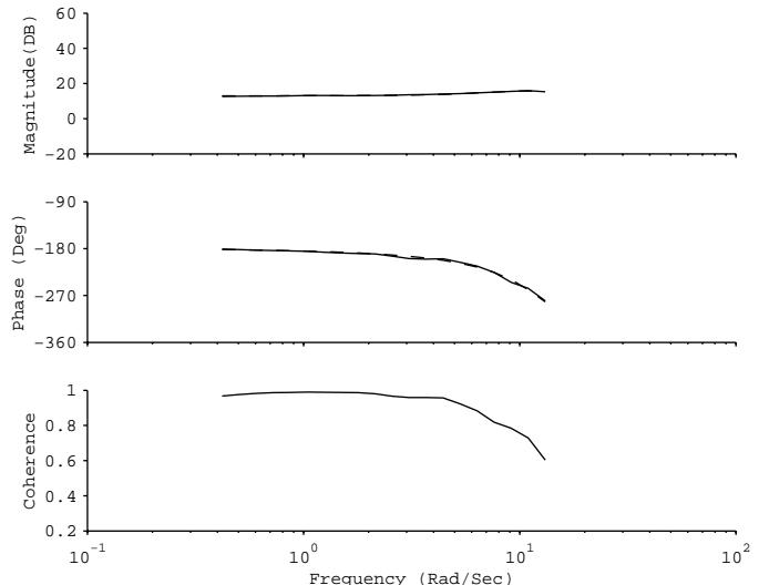
Fig. 17. Frequency-domain model fitting:  $\delta_{\text{rud}}$  to  $r$ .
