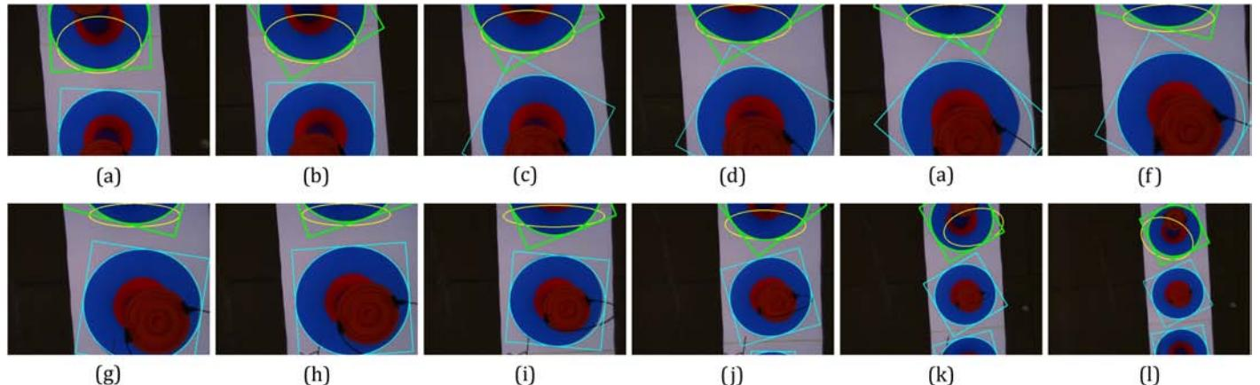
Fig. 26. Onboard images with the ellipse detection and tracking result.
