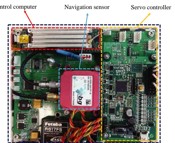
Fig. 8. Control hub with all hardware components attached.
