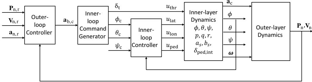
Fig. 18. Control structure of NUS<sup>2</sup>T-Lion.
