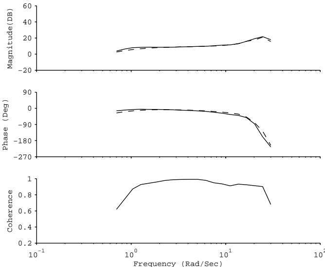
Fig. 15. Frequency-domain model fitting:  $\delta_{\text{lat}}$  to  $p$ .
