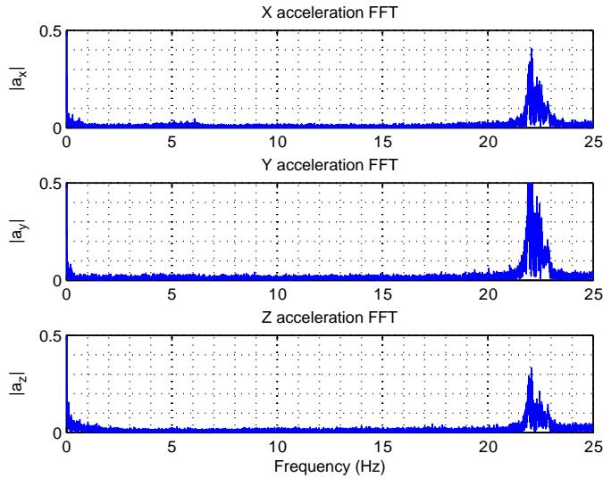
Fig. 11. Frequency analysis of acceleration without isolators.
