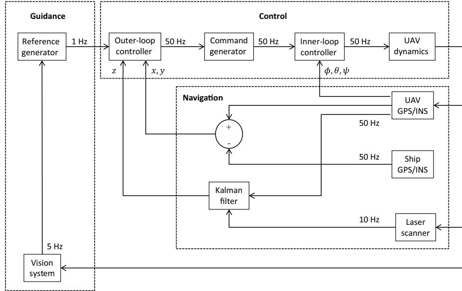
Fig. 13. Overall structure of guidance, navigation and control.
