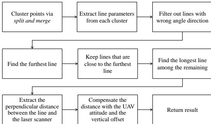
Fig. 20. Steps to compute height via laser scanner measurement.
