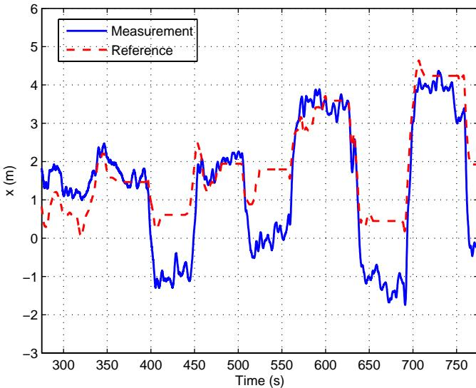
Fig. 32. UAV position response in the ship-frame  $x$ -axis.
