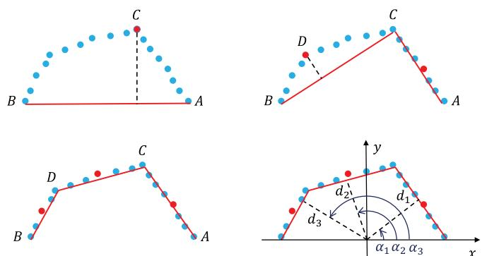
Fig. 19. The *split-and-merge* algorithm for line extraction.
