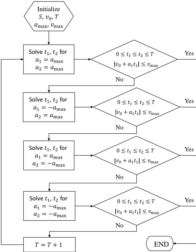
Fig. 28. Flowchart of the trajectory planning algorithm.
