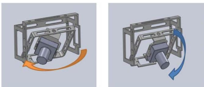
Fig. 9. Camera pan-tilt mechanism.
