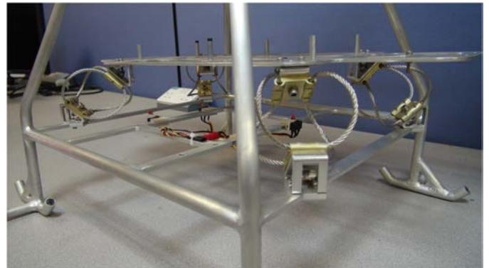
Fig. 10. Anti-vibration using wire rope isolators.
