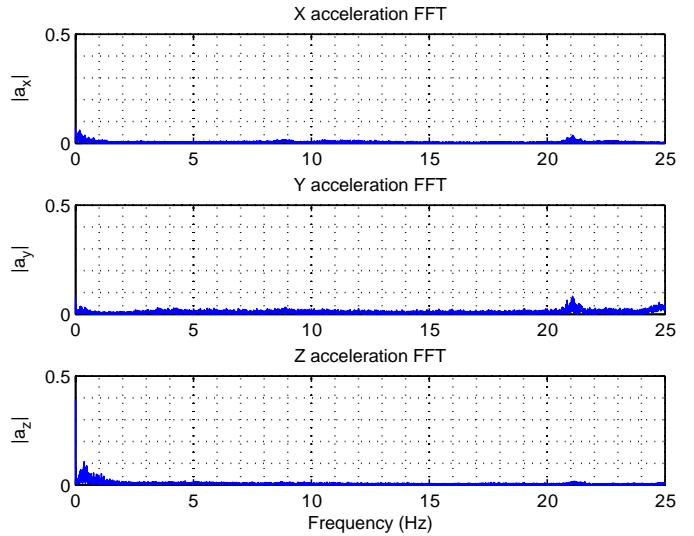
Fig. 12. Frequency analysis of acceleration with isolators.
