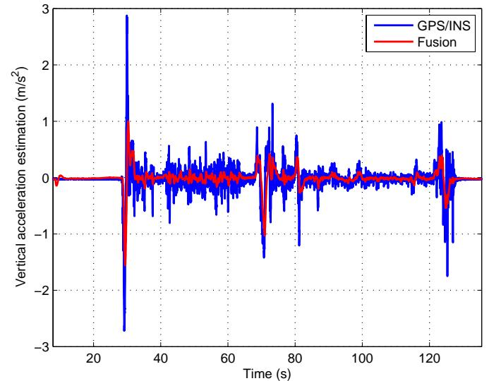
Fig. 24. Result of vertical acceleration estimation by data fusion.
