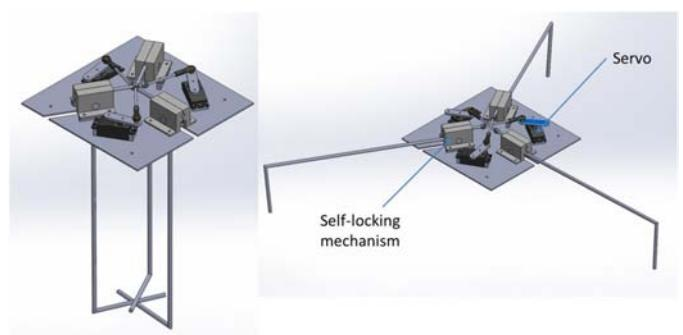
Fig. 5. Grabbing mechanism in closed and open configurations.
