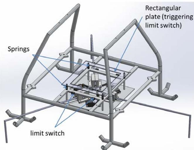
Fig. 6. Landing gear with bucket grabbing and load sensing functions.
