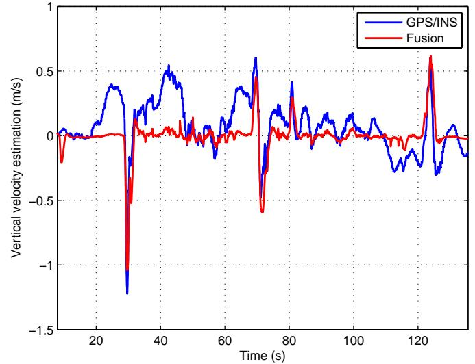
Fig. 23. Result of vertical velocity estimation by data fusion.
