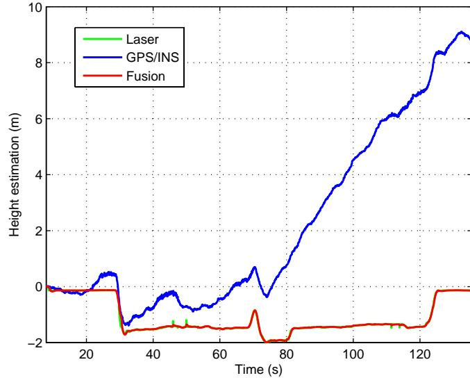
Fig. 21. Result of height estimation by data fusion.
