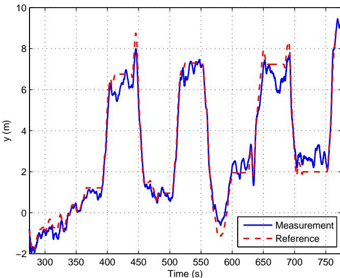
Fig. 33. UAV position response in the ship-frame  $y$ -axis.
