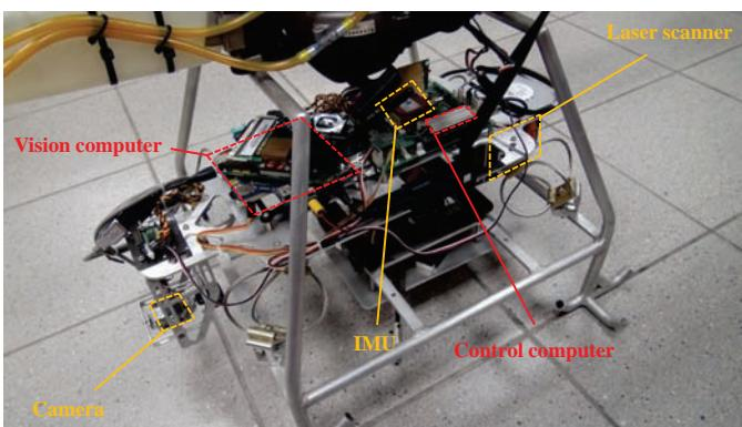
Fig. 7. Onboard avionic system of NUS<sup>2</sup>T-Lion.
