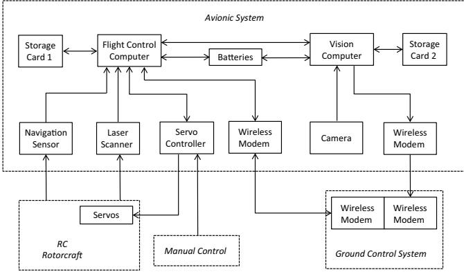
Fig. 4. Hardware configuration of NUS<sup>2</sup>T-Lion rotorcraft system.
