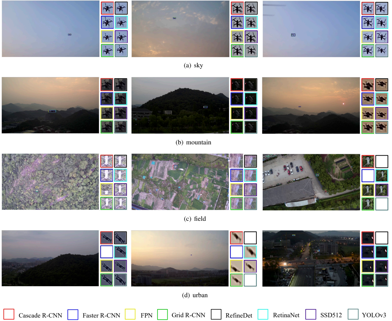
Fig. 2. Samples of images in the dataset and the corresponding detection results by the eight algorithms. The dataset contains four types of background scenes: sky, mountain, field, and urban. The detected areas by the eight algorithms are given right of each sample image with color-coded boxes. If the corresponding area is blank, it means that the algorithm does not detect any target UAV in this image.
