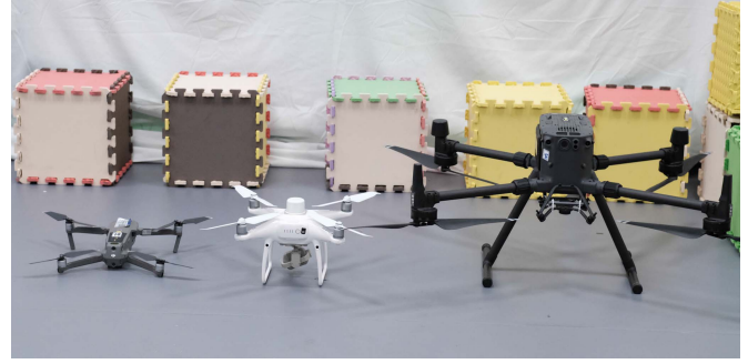
Fig. 6. Three MAVs in the dataset. From left to right, they are Mavic 2, Phantom 4 and M300, respectively. The indoor dataset contains Mavic 2, while the outdoor dataset contains all three MAVs.
