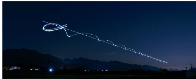
Fig. 1. Trajectories of the target and pursuer MAVs in one of our experiments. The target MAV moved with a constant speed of 5 m/s. The pursuer MAV executed the proposed bearing-only estimation and control algorithms. Each MAV has onboard lights. The photo was obtained by long-exposure photography.
